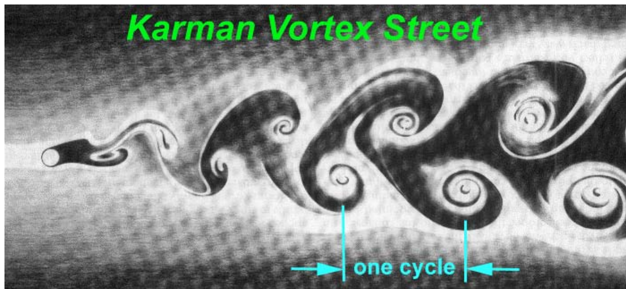
Figure 3. Vortex Shedding around a Spherical Body
